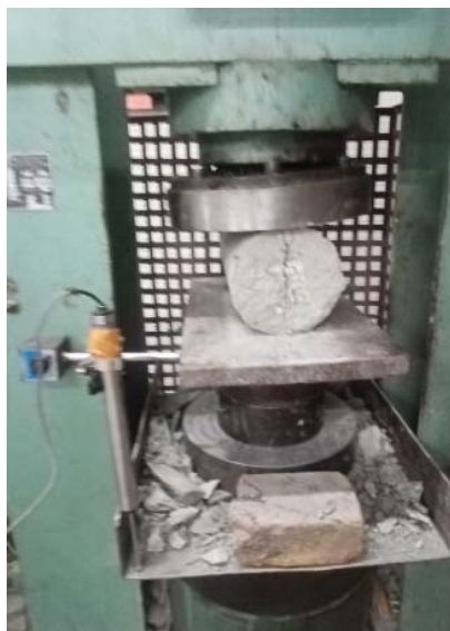
Figure- 18: Controlled Concrete Cylinders after split-tensile strength test
