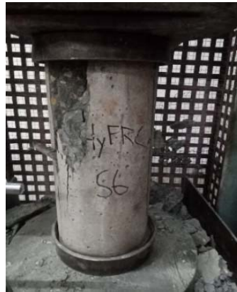
Figure- 13: HyFRC-S6 Cylinder after compressive strength test
