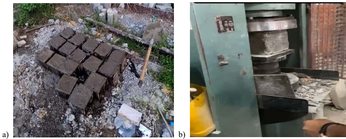
Figure 5: Cubes, a. casting of cubes, and b. testing of cube
