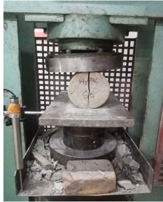
Figure- 16: HyFRC-S6 Cylinder after split-tensile strength test
