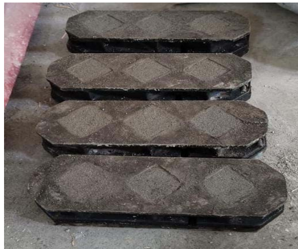
Figure 3: Mortar mix Casted in Moulds.
