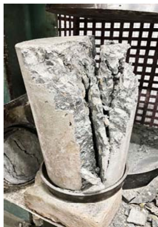
Figure- 15: Control Concrete Cylinder (CS) after compressive strength test
